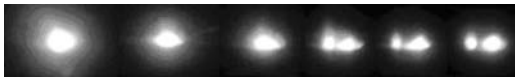
Fig. 6 Plasma shapes of hybrid welding with different standoff distances D_{LA}=1 mm, 2 mm, 3 mm, 4 mm, 5 mm, and 6 mm, respectively (see Ref. [18])
